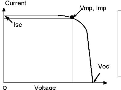
Plot of IV curve for a solar cell. Current times Voltage equals Power. Short circuit current (the current when the voltage is zero) increases in proportion to the incident energy (sunlight).
